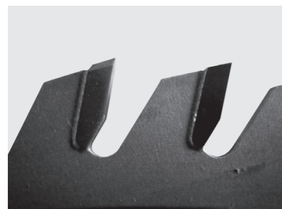
Tooth geometry trapezoid/flat tooth
